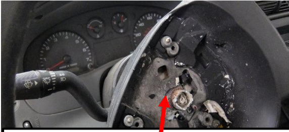
The steering wheel in the 2006 Ford Ranger belonging to Joel Knight. He was killed in December when the vehicle's Takata airbag ruptured after he ran into a stray cow in South Carolina.
