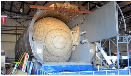
A look at an inflatable 32 ft long, 16 ft diameter device that could save tunnels from flooding.
