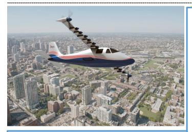
COMMENT #2 by author: For takeoff and landing, 12 smaller 9-kilowatt motors powering two-foot-wide propellers will kick in to blow extra air over the skinny wings to generate the necessary lift. For the X-57, the NASA researchers are designing narrower wings that are efficient during cruise flight. Thus, for sufficient lift on takeoff 12 smaller 9 Kw ...2 ft. diameter props are turned on to produce blowing air over narrow wings
