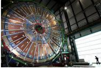
One station of the CMS Endcap Muon chambers built by a collaboration of US institutions, which play a major role in the triggering of the CMS detector.
