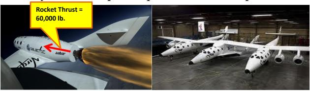
**INTRODUCTION:** As you can see in the picture at right SpaceShip2(SS2) is carried by a mother Plane(WhiteKnight) at 200 mph to 47,000 ft. where it is released and 60,000 lb thrust
