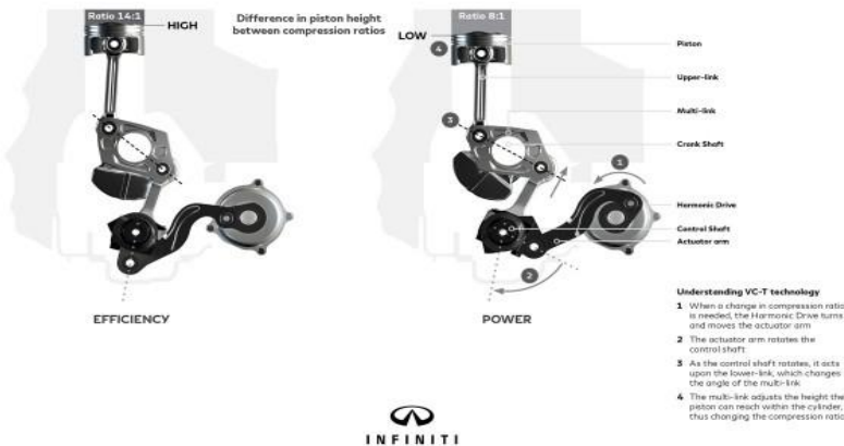
INFINITI VC-T ENGINE COMPARISON OF VC-T TECHNOLOGY IN HIGH AND LOW COMPRESSION RATIOS
