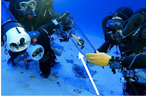
Divers collect fish with a portable decompression Chamber developed to help scientists study species from the ocean's mesophotic zone(130-490 ft. deep)
